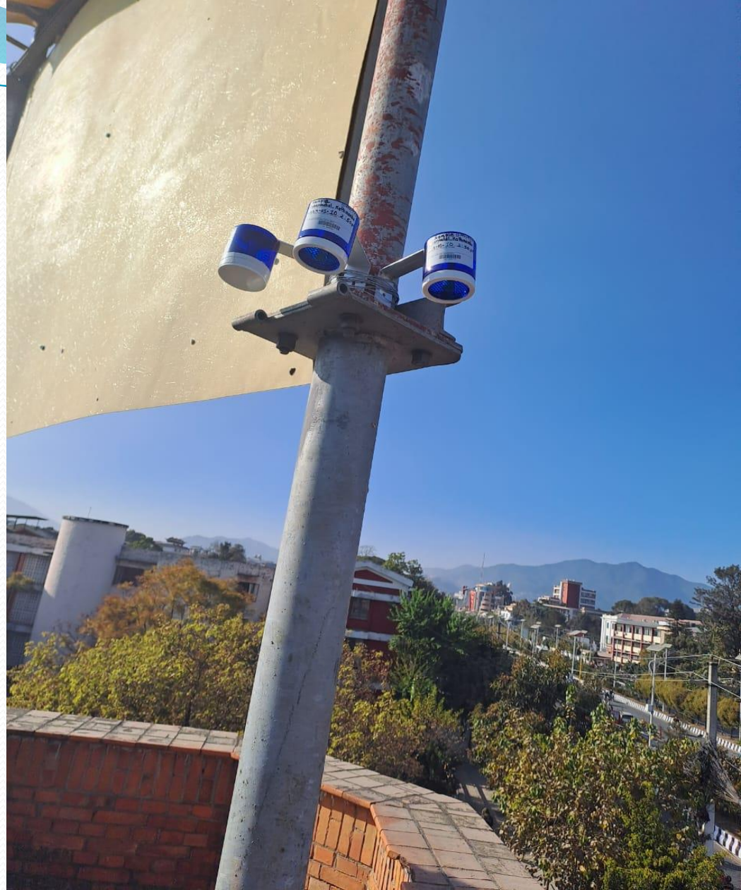
Mercury Passive Air Sampler (MerPAS)
